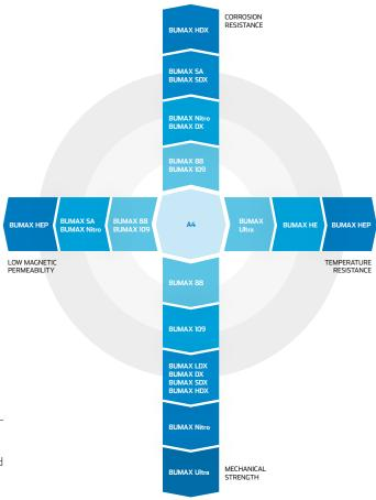
Stainless steel fasters have properties which make them attractive choices for a wide range of applications. It is essential to consider the required properties such as corrosion resistance, temperature resistance, mechanical strength and magnetic permeability. Correctly chosen material will guarantee a trouble-free life time and low life cycle cost.
